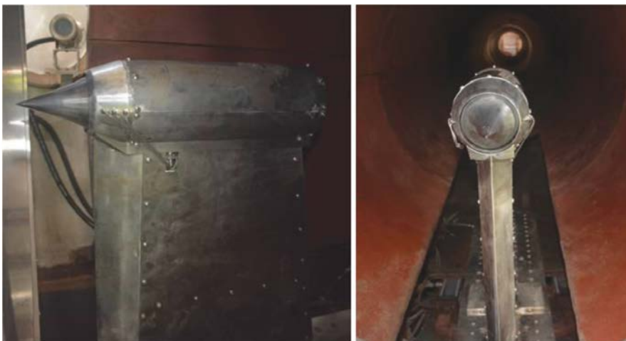
Ground tests of a hydrogen-fueled continuous-rotating detonation ramjet at Mach 4.5 and simulated 18.5-km altitude indicated positive thrust was obtained (see page 54).
