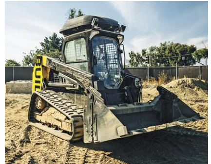
NO OPERATOR REQUIRED Built Robotics’ skid-steer package uses LIDAR and GPS to navigate sites.
