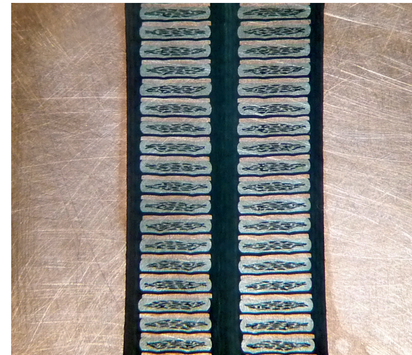
MAGNESIUM DIBORIDE MASH: Filaments of the superconductor magnesium diboride are encased in ribbonlike support structures of copper and other elements. The ribbons are then carefully wound into a "racetrack" shape to form the turbine's high-power electromagnets.
