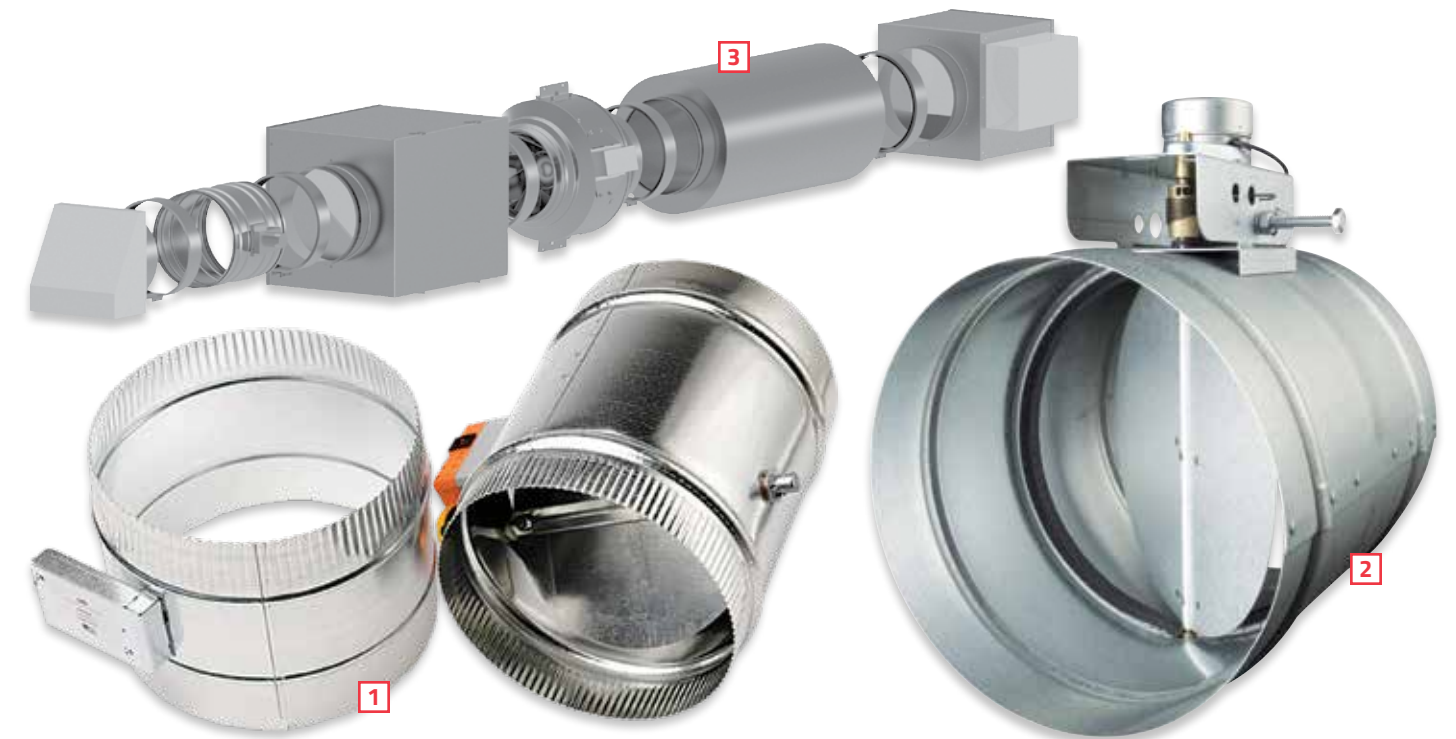
Editor's Note: Examples of makeup air solutions include: 1 The Residential Makeup Air System (RMAS) from CCB Innovations includes an air flow sensor mounted inside a standard duct coupling, which signals a motorized damper in a second coupling to open when air is flowing and close when air flow stops. 2 Broan's direct-wire, synchronized Automatic Make-Up Air Dampers work with specific company range hoods, operate automatically when the range hood is activated, and are compatible with whole-house ventilation systems. 3 The automated Makeup Air System (MUAS) from Fantech includes an intake hood, shut-off damper, filter, fan, duct silencer, and optional heater; available models handle air flow up to 2,000 CFM.
