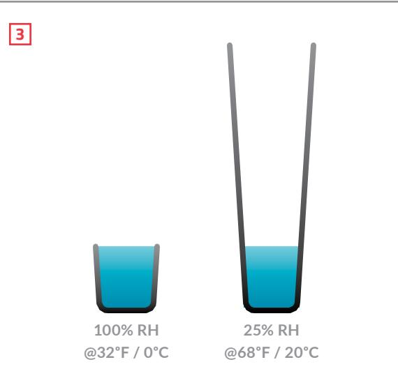
When we ventilate a house with cold, moist air, the RH drops as the air warms. For example, if the outside air is 100% RH at 32°F, the RH drops to 25% when the air reaches room temperature.
