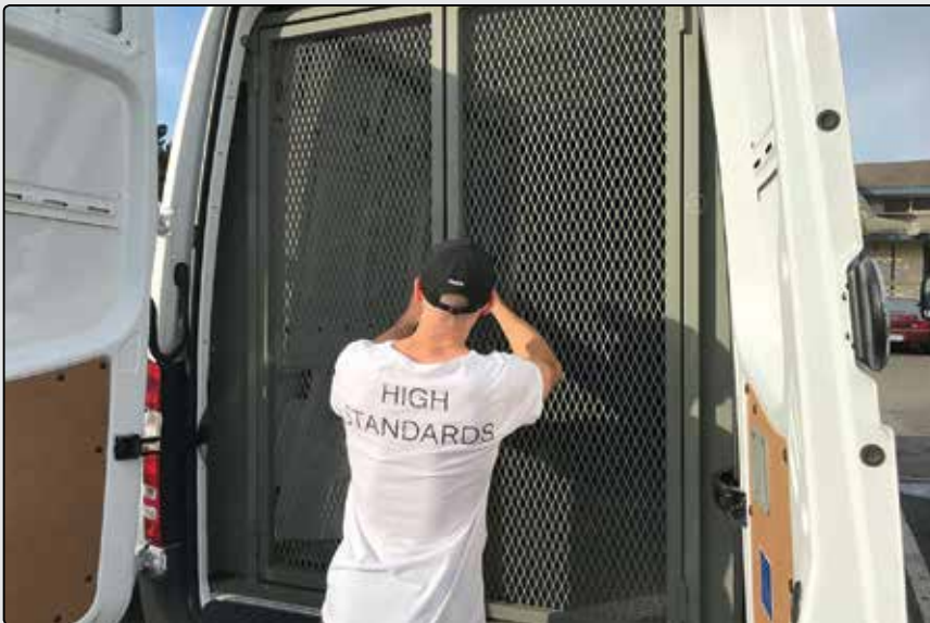
This attached caging at the back of a Nabis-owned Nissan NV200 is part of what’s required by the California Bureau of Cannabis Control’s cannabis-transport regulations. Nabis CEO Vincent Ning says the regulations also led to outfitting vehicles with security cameras, alarm systems and GPS units.
