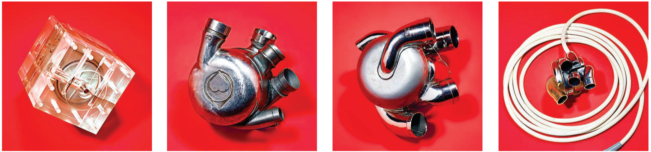
EVOLUTION OF AN IDEA: Timms came up with the original concept of an artificial heart with a centrifugal pump in 2001 and has been developing the technology over the past 18 years. The first concept model [left] tested the hydraulic feasibility of the design, with a single rotor pumping fluid in two directions. Later prototypes [middle left and right] were used for the crucial tests in cows. The final design [right] is more tailored for human anatomy.
