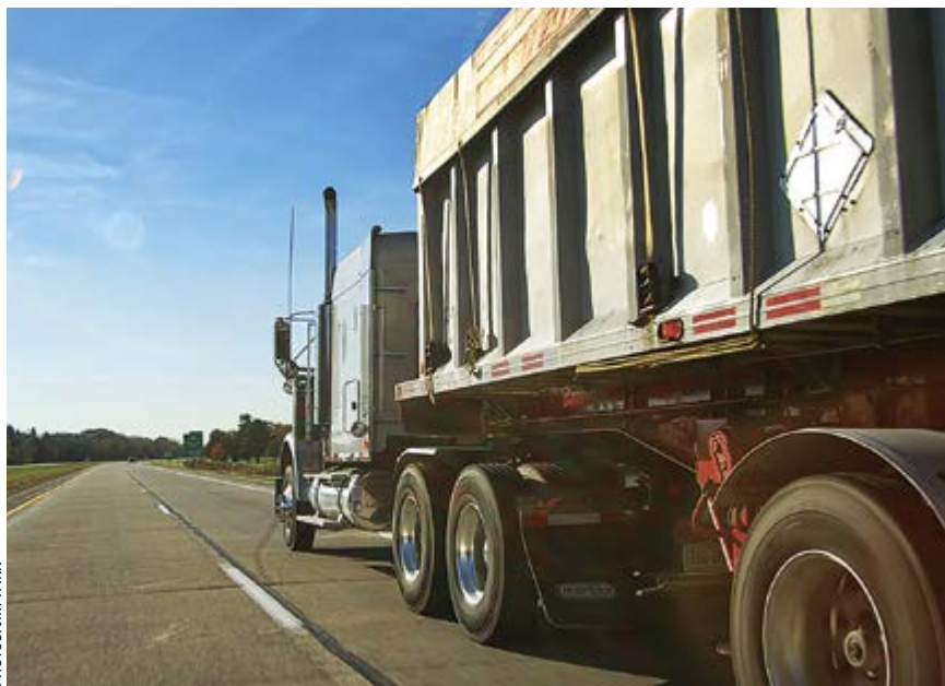
Lane-keeping assist steering technology will actively nudge the truck back into the lane if the driver begins drifting across the line.
