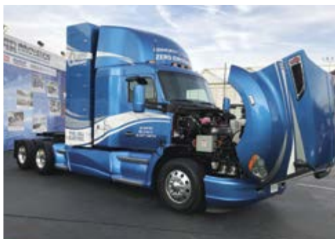
Kenworth and Toyota are partnering on a fuel-cell-powered Class 8 tractor for regional hauls of up to 350 miles.
