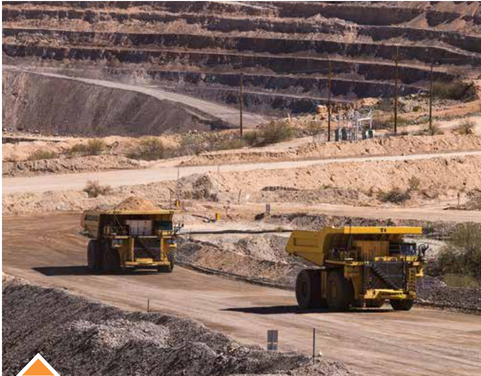
Komatsu Autonomous Haulage System-equipped trucks have moved more than 2 billion metric tons of material in the mining sector.
