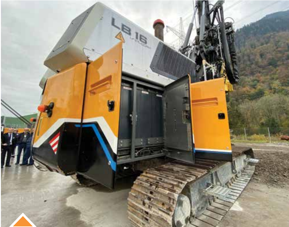
Future now: Liebherr unveiled its LB 16 electro-hydraulic drive drilling rig this fall in Germany, designed to be charged overnight after a 10-hour work cycle. Servicing and repairing such machines will likely be one future technician skill adaptation.
