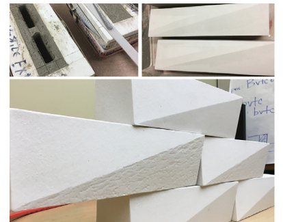
FIGURE 11. Handcrafted terra cotta prototypes
