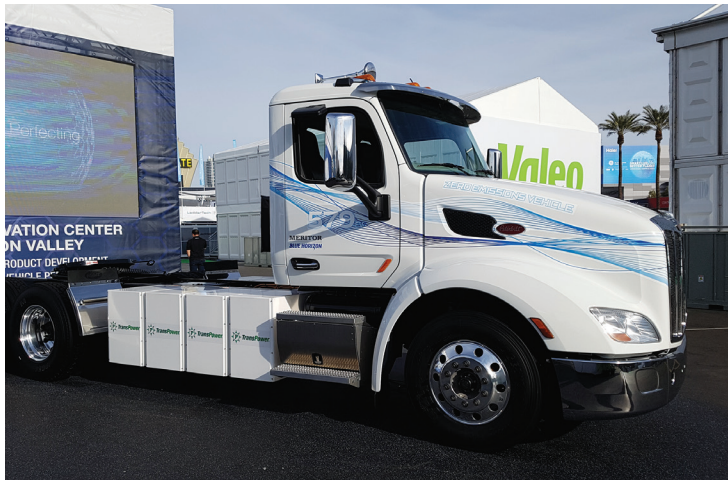
As chassis integration evolves, electric trucks will become lighter and less expensive. Wheel-end motors could replace traditional drive shafts and differential axles.
