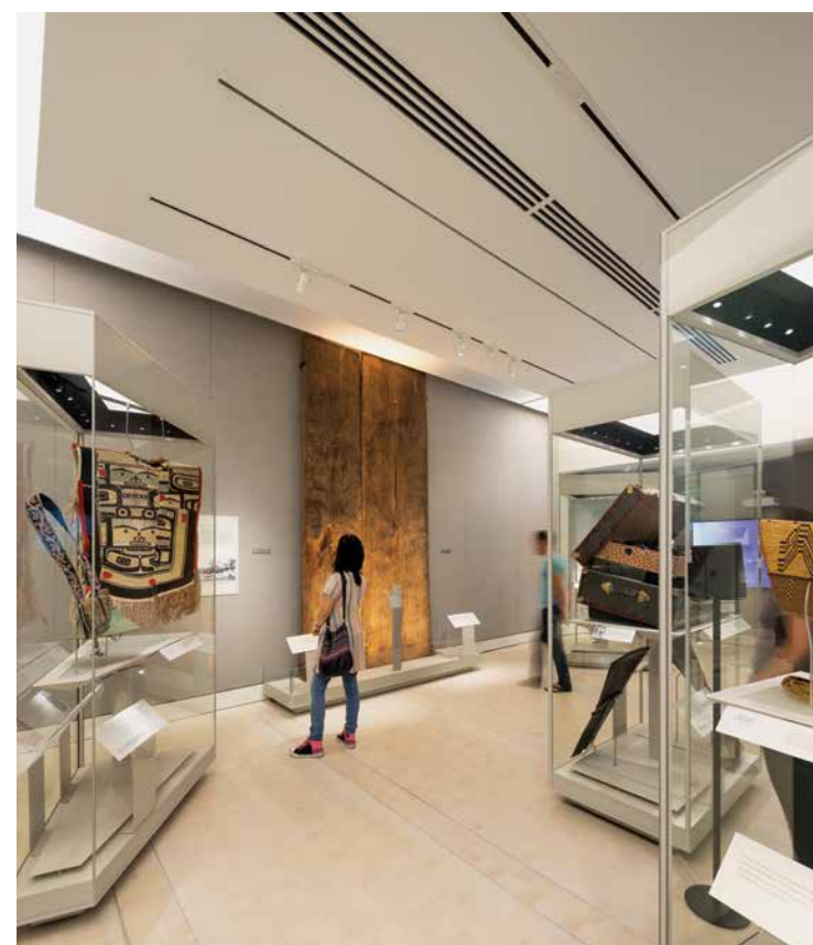
A new gallery at the Museum of Anthropology at the University of British Columbia in Vancouver (opposite and both above) relies on tunable-white LEDs to mimic actual daylight conditions in real time. A rooftop sensor reads outdoor lighting color and intensity, and a control system adjusts the room's illumination accordingly.
