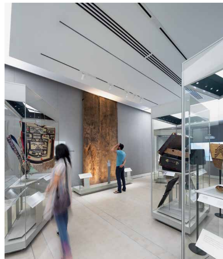
A new gallery at the Museum of Anthropology at the University of British Columbia in Vancouver (opposite and both above) relies on tunable-white LEDs to mimic actual daylight conditions in real time. A rooftop sensor reads outdoor lighting color and intensity, and a control system adjusts the room's illumination accordingly.
