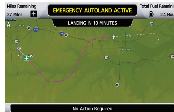
Cockpit displays keep the passengers "in the loop" by showing where the aircraft is located, what divert field has been selected, how the aircraft will be maneuvered and when it will arrive at the airport.
